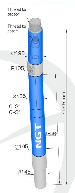
Bearing section S–195.NGT.M4 is a new short bearing section featuring enhanced operation life. The bearing section is used in PDM power sections of 195 mm diameter and for drilling oil and gas wells with 215.9-269.9 mm rock and PDC bits.
