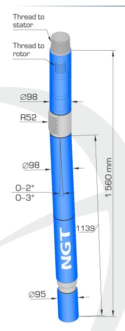
Bearing section S–95.NGT.M1 is a new short bearing section featuring enhanced operation life.
